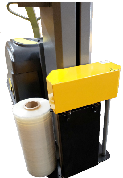
Pre-stretch carriage saves up to 60% on film costs
