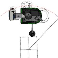
Power the machine on by turning the on switch and holding for 3 seconds. To begin wrapping pallets, position the machine next to the desired pallet with the controls located on the handle. Be sure there is an additional 56" clear around the pallet for the machine to operate. Raise or lower the height of the guide wheel as needed to allow smooth rotation around the pallet.
