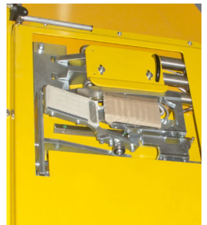
Automatic Sealing Unit: Attaches, Cuts, & Hot welds the film tail
