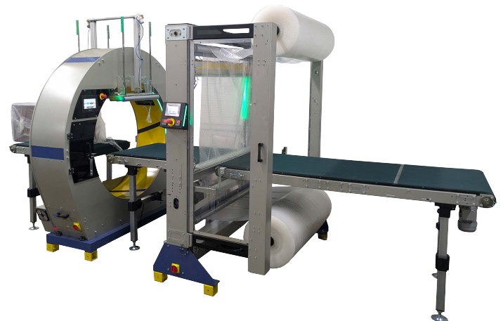
OWM-DPBP125 with driven conveyors & top presses (optional).
