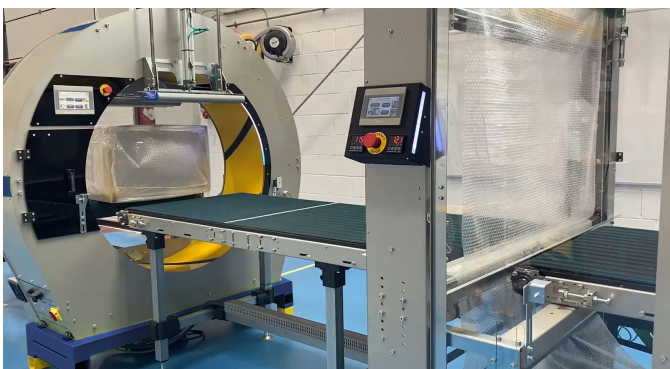
OWM-DPBP125 with driven conveyors & top presses (optional).
